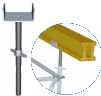
7) Head spindle "U" • opening width 160 mm • supporting length 150 mm • boreholes for fixing formwork girders • max. spindle travel 0.45 m
